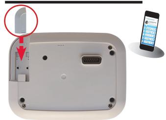
The optional Wi-Fi module enables the controller to be remotely monitored and accessed anywhere within range of your home wireless network device, and can be remotely controlled with a smartphone
